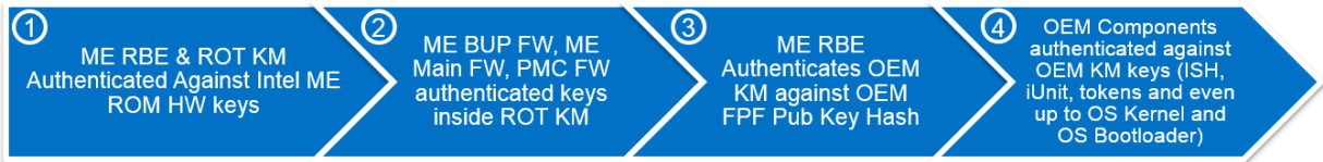
Figure 2: Platform Chain of trust extended from Intel HW Root of Trust (ME ROM HW)
